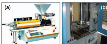
Figure 26.9 Equipment employed in the production of the blends: (a) twin-screw extruder; (b) hot-plates press.
