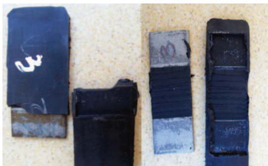
Figure 5.34 Photographs of samples which failed by cohesive failure based on CV system.
