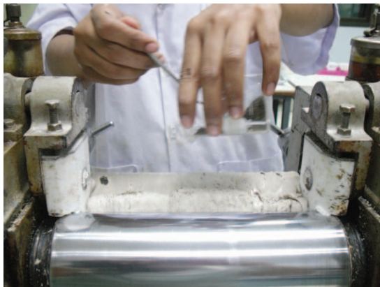
Figure 13.17 Preparation of rubber composite using a two-roll mill (author's experiment).
