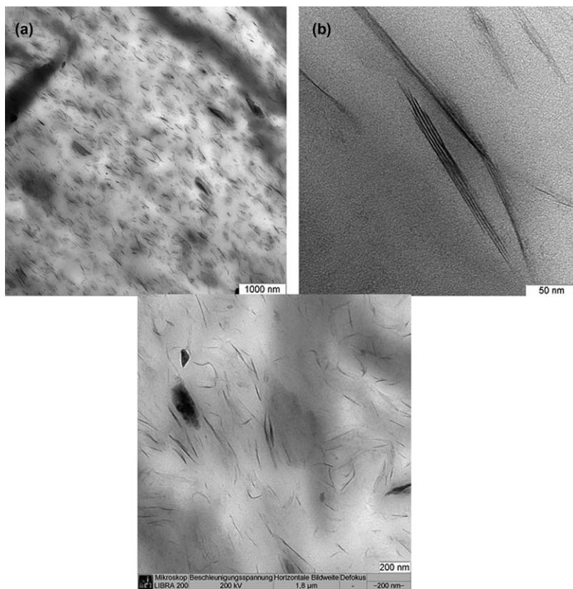
Figure 8.17 Different TEM images of NR nanocomposites with 10 phr of EOMt; different scale length. (Reproduced with permission of Elsevier Ltd.)
